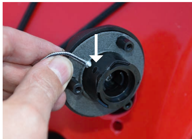
23. Feed the end of the line through the outer hole on the skeg control unit. First make sure that the hole inside is aligned to the outer hole.
