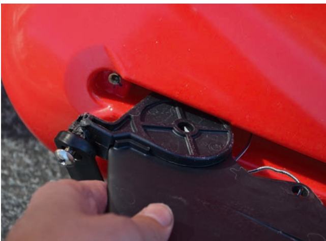
16. Put the skeg and skeg line into the new replacement rudder.
