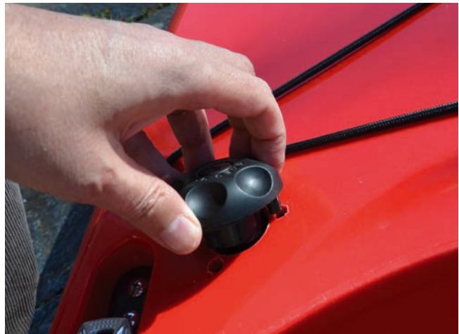
27. Push the control unit through the holes and keep pressure on it, while aligning the bottom of the unit inside the back section. Again this will be easier to access, if the section is standing up.
