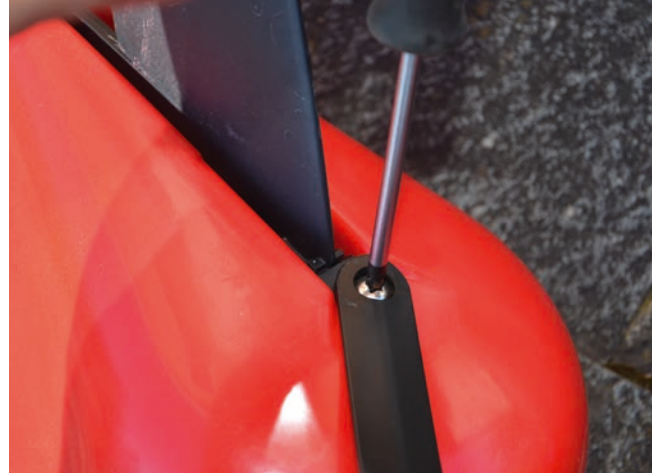
13. Now you need to take out the skeg by unscrewing the large screw holding the rudder foot plate and skeg on to the rudder.
