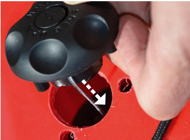
26. Place the control unit over the hole on the deck. Make sure the hole, where the line comes out, is facing backwards to line it up with the skeg tube inside.
