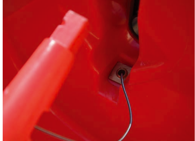
19. Feed the line into the hole and bring the rudder into position while continuing to feed the line into the hole.
