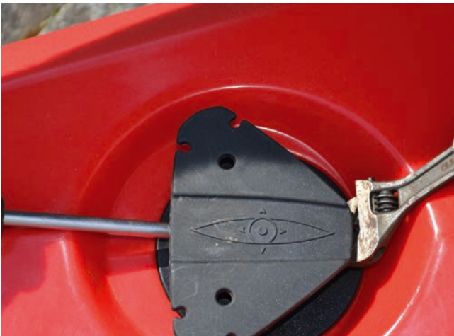
8. Hold the nut with the wrench and unscrew the screw on the other end.
