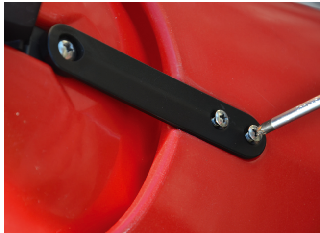
21. Fasten the Rudder foot again. Fasten the first screw halfway before putting in the second screw. Screw them on firmly.
