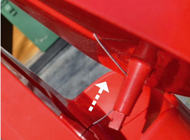
12. Pull out the whole rudder including the skeg out of the hull, the pull up line for the skeg will follow out.
