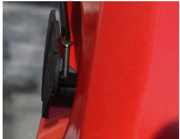
9. The crew is quite long and needs to be unscrewed all the way until it comes out.
