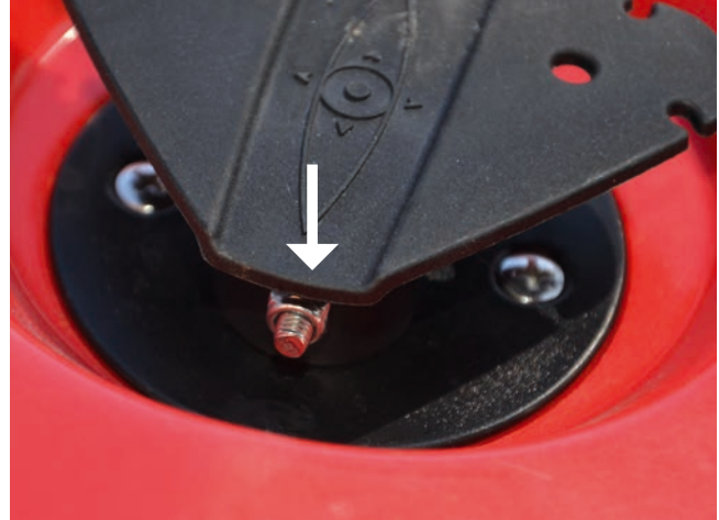
7. After this you need to undcrew the rudder head from the rudder. You will need the longer screw driver and wrench to undo the screw holding them together.
