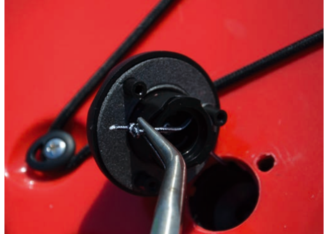
7. To make the line shorter, you should pull out the line with the plyer and undo the knot
