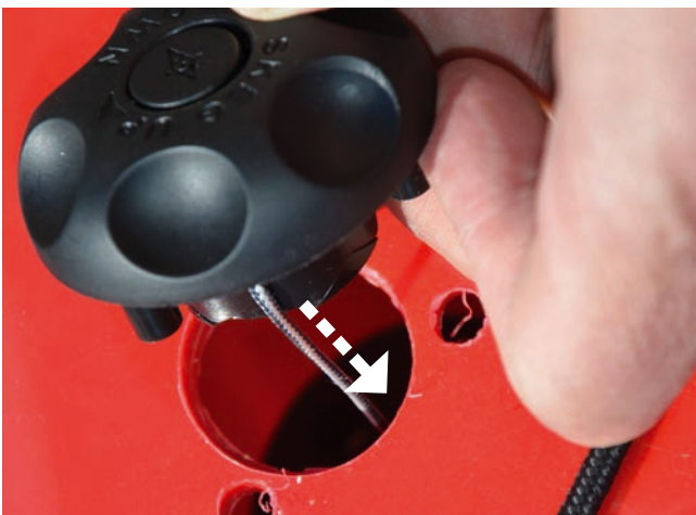
10. Place the control unit over the hole on the deck. Make sure the hole where the line comes out is facing backwards to line it up with the skeg tube inside.
