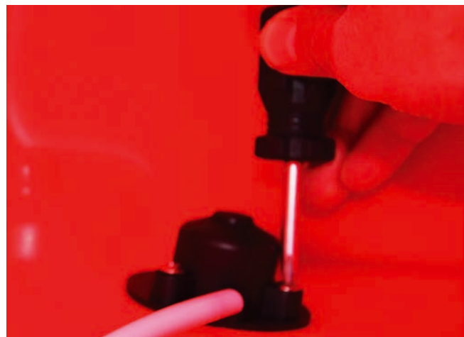
11 Push the control unit through the holes and keep pressure on it, while aligning the bottom of the unit inside the back section. Again this will be easier to access if the section is standing up. Screw on the 3 screws inside the section. The skeg should now be able to come out by itself.
