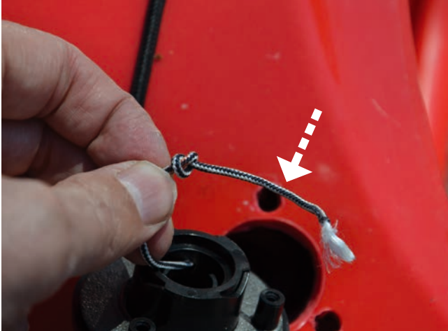
6. A different reason could be that there is too much line after the knot, which also might jam the mechanism
