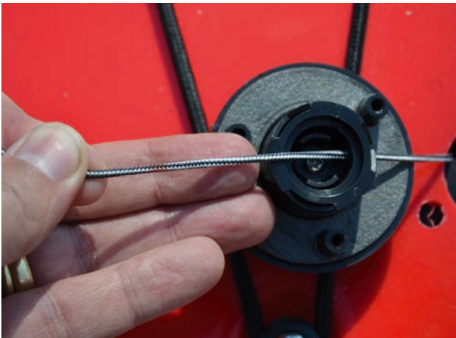
8. Pull the line as much as possible (make sure the skeg is up in the rudder, and make a new knot as close to the unit as possible
