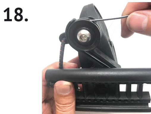
18. After threading the line through the channel, turn the slider around and put the pedal line through the pedal and pedal wheel as shown in the image above.
