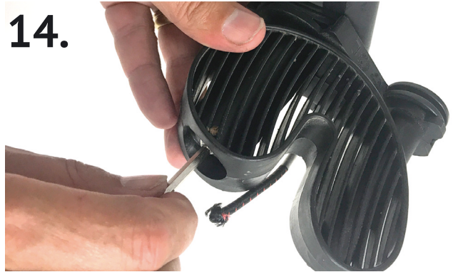
14. Screw in the screw lightly at first to make it catch on the nuts threads. Tighten the screw lightly, do not tighten hard!
